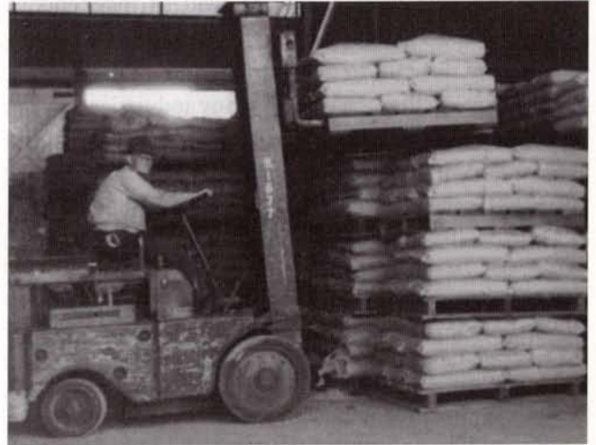
50 year old internal combustion forklift - no overhead safety guard, basic, central lift cylinder, manual, no power steering, noisy.
