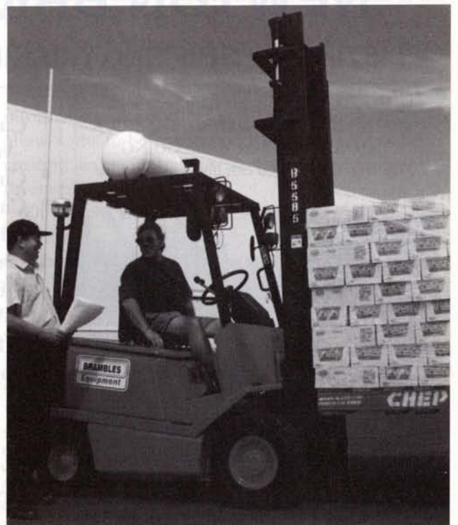
Current model internal combustion, ergonomic control, overhead safety guard, suspension seat, wide view mast, automatic quiet, power steering
